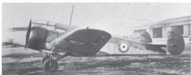
Developed for spinning trials and also to study the effects of twin fins and rudders, Oxford N6327 was a one-off conversion and spent most of its time, as shown here, at the Royal Aircraft Establishment, Farnborough.
