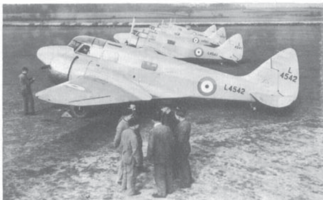
This early line-up outside the factory at Portsmouth was taken in March, 1938. The aircraft are painted yellow overall with natural metal cowlings and only the farthest aircraft, L4544, has a dorsal turret although they are all Mk. Is. (Photo: "Flight" 15455S)
